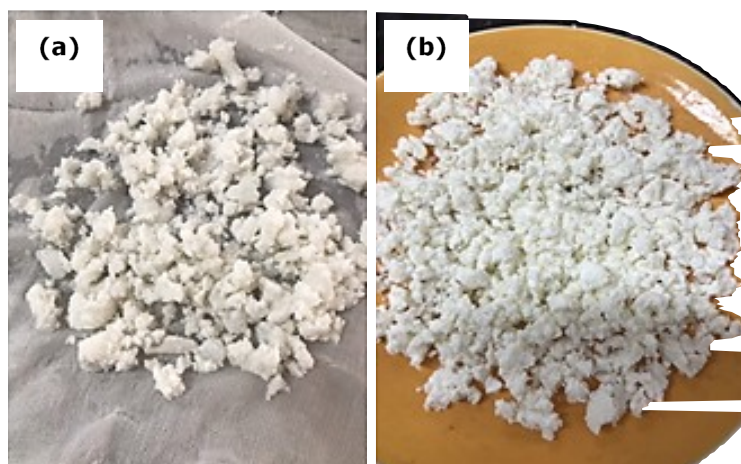
Figure 2: MIPs (K-g-PAA) wet (a) and dry composite (b).
